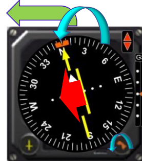
Intercept Radial 180° Inbound Track 360° to FIX
